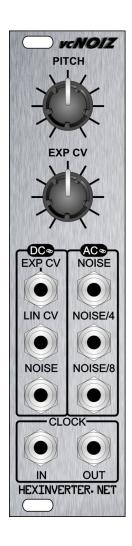
Pitch Control -- This controls the base frequency of the noise VCO, just like any other VCO. Express yourself using this control while playing live for some awesome crunchy pitch sweeps! Turning the pitch all the way up will produce white noise at the AC NOISE output. Turning it all the way down will produce sub-audio clicks and pops which are suitable for use as random gates and to trigger events in your system.
