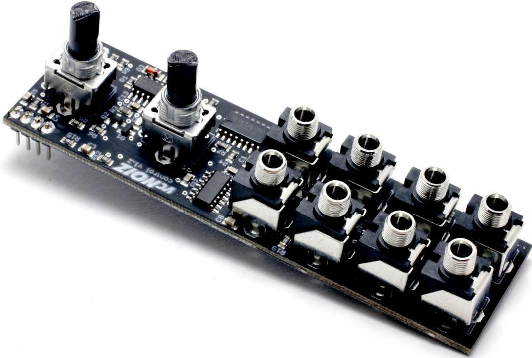
Next, remove the protective plastic from the eurorack panel and install it onto the control surface PCB. Finger tighten two opposite nuts onto the jacks. **Don't use a tool to tighten the jacks, and do not solder any of the components yet!**
