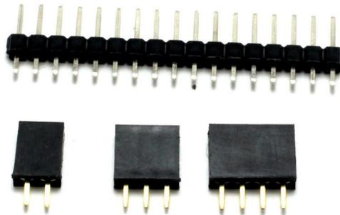
Snap a 4pin, 3pin and 2pin section off of the longer male header:
