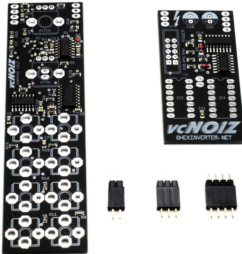
Now, install but do not solder the header assemblies into the control board, like this:
