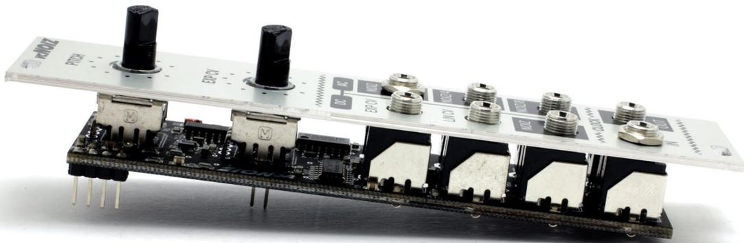
Now is when you have to be really careful. Flip the assembly over and **solder one leg only** of each of the components on the control surface PCB.
