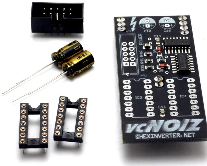
Solder in the components, beginning with the two 14pin IC sockets. **Make sure the notch is aligned with the PCB's graphics.**
