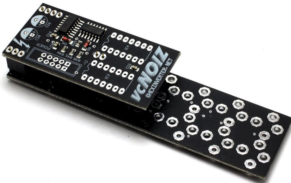
Now, being careful to keep the headers straight, “tack” one pin of each header in place with the soldering iron. Inspect your work and reheat any soldering joints while adjusting the PCBs to ensure that the assembly goes together aligned in a straight fashion.
