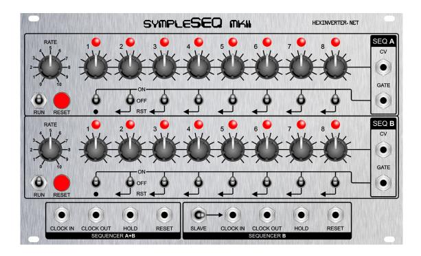
RATE CONTROLS - These control the rate (tempo) at which the sequencer's internal clock advances the sequencer/s at.
