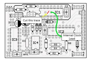
**Step 2:** Prepare the logic board for the 5V clock level input conversion.
