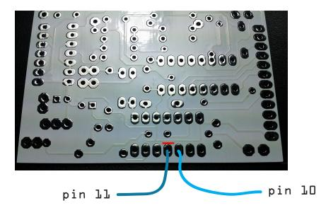
With your new internal clock lead and these two pins of the 40106 being brought out to wires, you are now ready to begin putting the panel wiring together!
