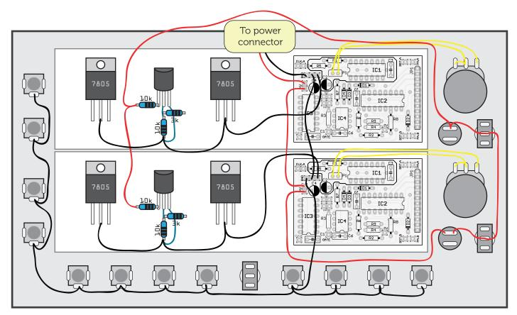
**Step 8:** Almost there! Finish off by adding the CV/Gate wires and soldering the .01uF capacitors across the switches' terminals. Pay attention to the resistor values used, of course.
