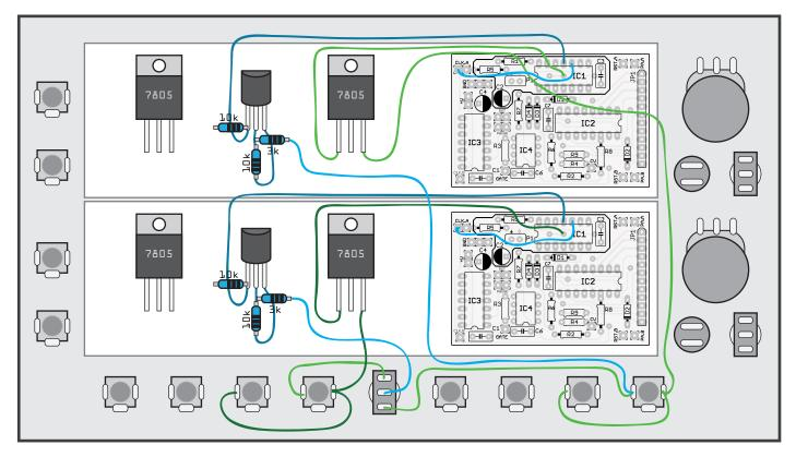
**Step 5:** Wire the reset circuitry, adding diodes where indicated. You may find that you can go straight from the button to the logic board with only the diode leads!
