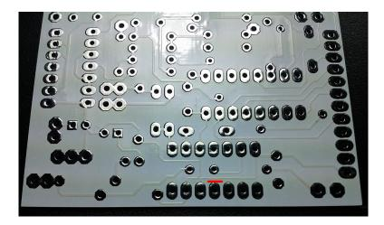
Now, solder on two wires to the two pads of the 40106 on the bottom of the logic board, as per the schematic. Take note of which one is pin 10, and which is pin 11. Using different coloured wire here is a good idea since the bottom of the logic board is not as visible when installed in the module.
