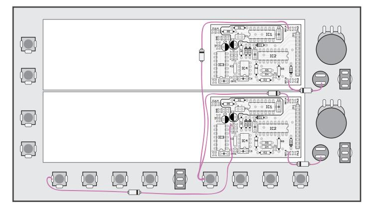
**Step 6:** Wire the pause circuitry, adding diodes where indicated. You may find that you can go straight from the button to the logic board with only the diode leads!
