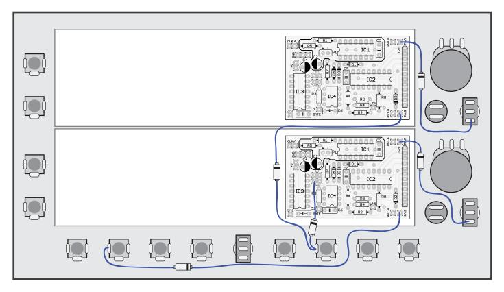
Step 7: Wire the rate control potentiometers and power connections
