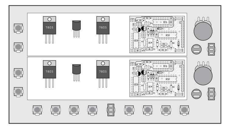
**Step 4:** Wire the clock signals as indicated, using standard SPDT ON-ON type switches and switching 1/8" jacks. Be mindful of resistor values and insulate anything you are concerned about shorting on the back of the control board. Leave the unconnected resistors hanging for now. We'll deal with them later.
