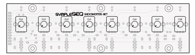
Install the 8 board mount potentiometers in their places, starting with the outer mechanical posts and adjusting them using the "tack method" as necessary to make them perfectly flat on the circuit board. It is crucial that they are aligned accurately so as to go through the panel in the
