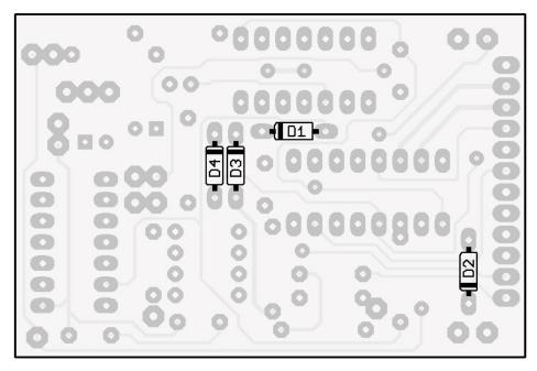
Next up is the diodes. Be careful not to apply heat for too long, as diodes can be damaged from excessive heat. Make sure that they are installed in the correct direction. The band on the diode is the negative side, and should be installed on the side with the band on the board silk-screen.
