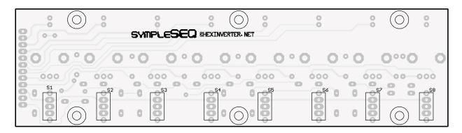
The switches have a flattened edge on one side of the post that you may wish to orient the same on all of the switches for aesthetic reasons. The switches themselves are uni-directional, so exact orientation does not matter. It's up to you whether the flattened part points up or down.
