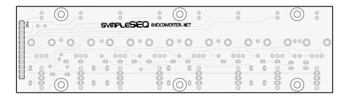
Install the female 12 pin header on the OTHER side of the board (ie: if you are looking at the board from the component side, the header should be facing away from you on the other side). This will mean that the logic board can "plug-in" from the back.
