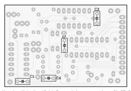
Now, install the four ICs' .1uF ceramic bypass capacitors, C1, C3, C6, C7
