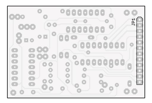
The last soldering step is to install the male header into the OPPOSITE side of the board. By doing this, you are making it so that the logic board will plug in to the back of the control board. So, just to make that clear: when you are looking at the component side of the board we have been working on, the header should be facing AWAY from you on the other side of the board when installed correctly.
