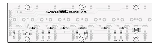
Install and solder the 16 diodes onto the board, again making sure that they are installed the correct way. Things will not work properly if they are installed incorrectly.
