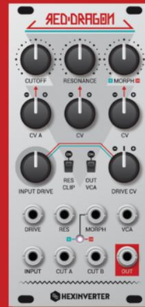
Turning the RES CLIP on clips the resonance feedback and produces different tones at high resonance settings.
