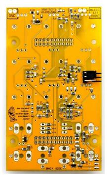
• The headers that connect the PCBs together can now be installed. The female headers are best installed on the Main PCB and the male headers on the Control PCB. Connect the two boards together and then solder the headers, making sure that the two boards' mounting holes are lined up nicely.
