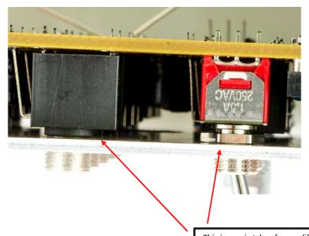
This image is taken from a different build to illustrate the way the switches and jacks should be flush against the panel (since you cannot see the switches easily to illustrate on the Mutant Snare, due to their location)
