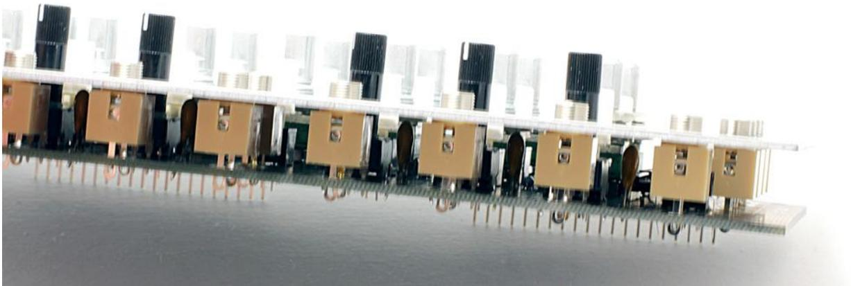
Once you are happy with the way that everything is seated, go ahead and **start soldering all the pins** of the potentiometers and switches. There are a LOT of pins to solder so take your time and don't miss any!
