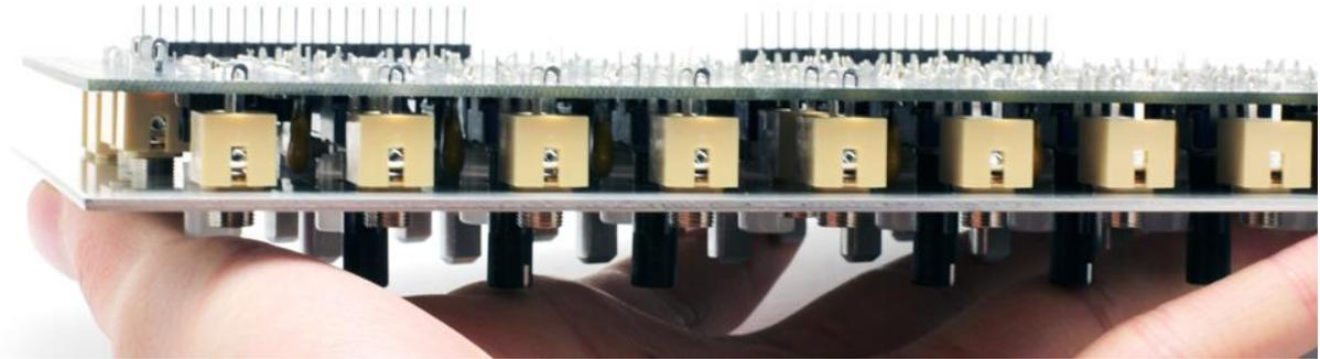
Keeping the panel upside down, you can **solder the legs of each jack** so that they stick up from the PCB when you flip it back.
