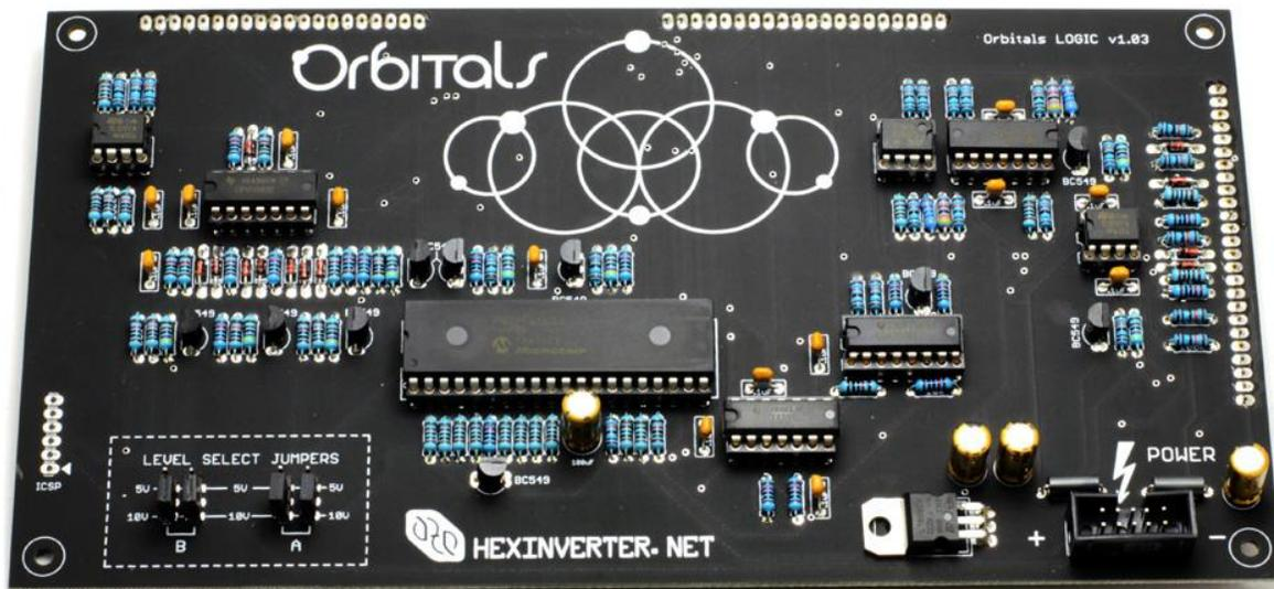
**Now you are done the actual electronics part of the assembly!** I highly recommend going over all of the backs of the PCBs one more time and making sure there are no shorts or missed soldering points. Once you put the PCB stack together and the panel on, it's pretty daunting to have to take it all apart again to fix a mistake. So, do it right the first time by **checking your work over now!**
