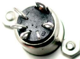
Attach the panel back onto the control PCB and then solder the wires to their respective numbers on the MIDI connector, passing the cable through the hole on the control board.
