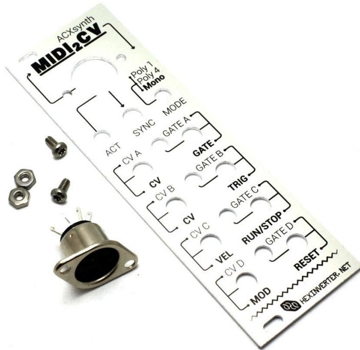
Using the two shorter machine screws with nuts and a Torx 10 (aka: T-10) screwdriver, affix the MIDI input jack to the panel.
