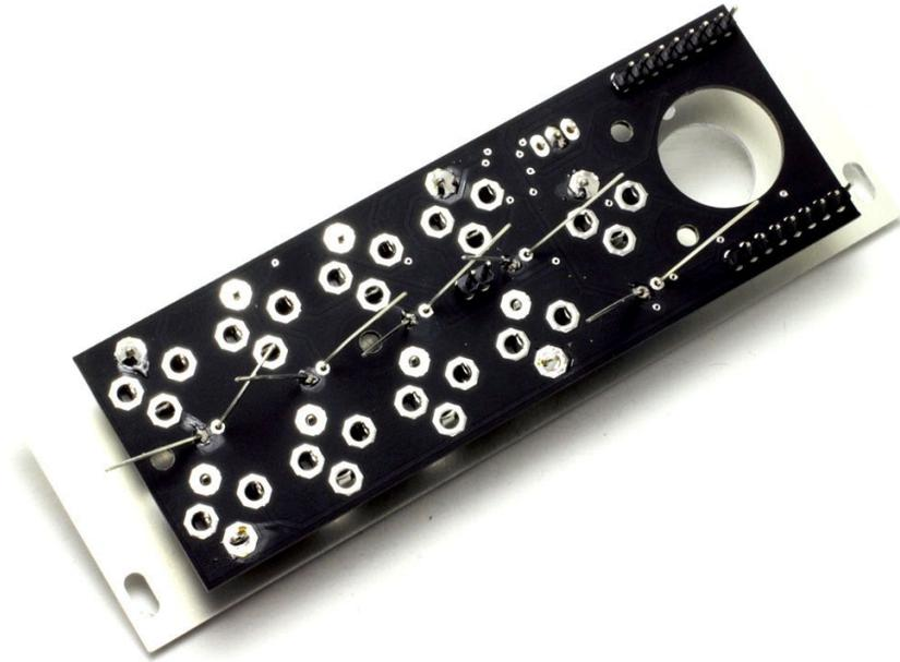
Now adjust the switch nut so that it is the same height to the panel as the jacks.
