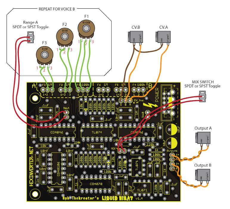
When MIX SWITCH is toggled up, Output A outputs a mix of Voice A+B
