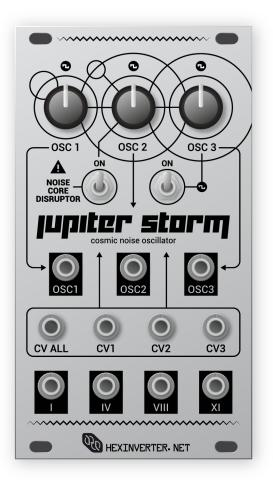
OSC1/2/3 Controls -- These knobs control the base frequency of each of the square waves in the Noise Core. A lot of change in sound can be experienced simply from playing with these controls.
