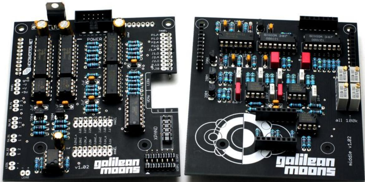
**Now you are done the actual electronics assembly!** I highly recommend going over all of the backs of the PCBs now and making sure there are no shorts or missed soldering points. Once you put the PCB stack together and the panel on, it's pretty daunting to have to take it all apart again to fix a mistake. So, do it right the first time by checking your work over now!
