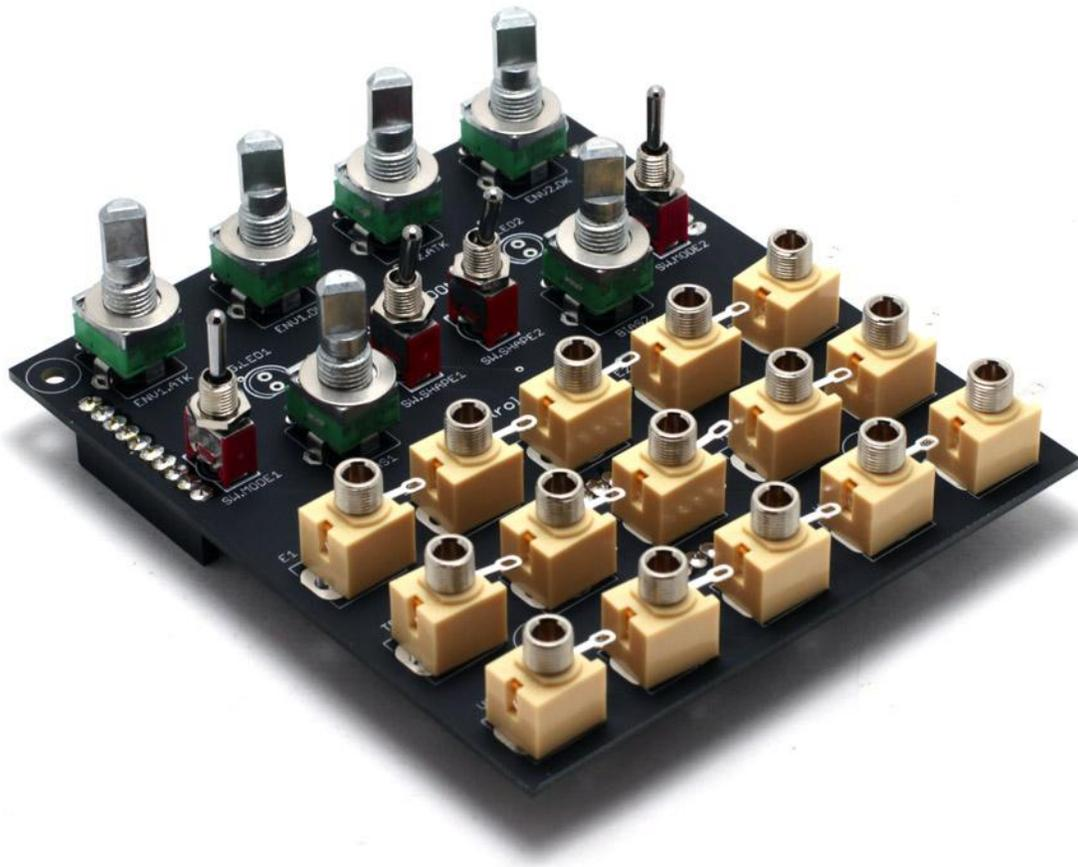
Remove the protective covering from the panel and install it on the loose-fitting control board components. Screw on the nuts for the potentiometers only. **DO NOT SOLDER ANYTHING YET!**
