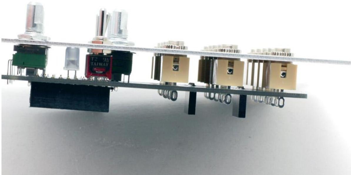
***Make absolutely sure that everything is positioned nicely***, then go ahead and start soldering the control components in place!
